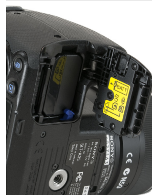
Figure 1-19: The blue lever holds the battery in place.
