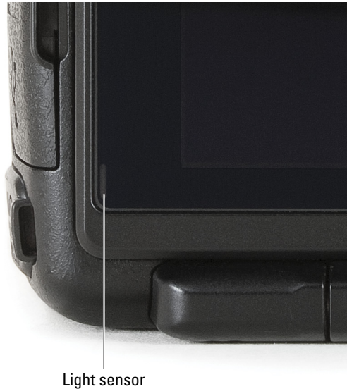
Figure 1-7: The sensor helps the monitor stay bright.
