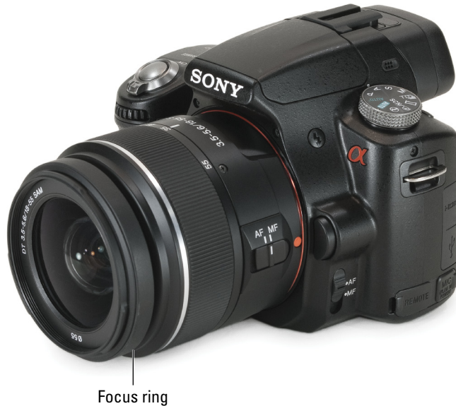
Figure 1-15: The focus ring is all the way at the end of this lens.
