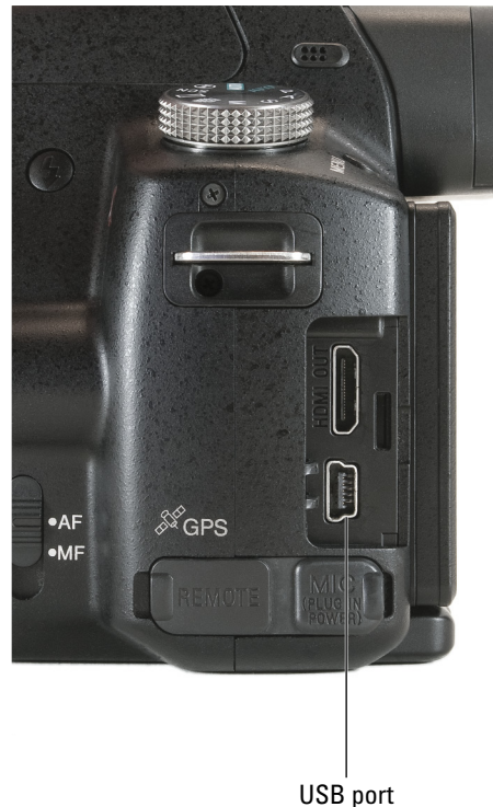
Figure 6-4: Insert the small end of the USB cable into the bottom port.
