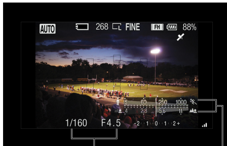
Numeric display of shutter speed and aperture Graphical display of shutter speed and aperture
