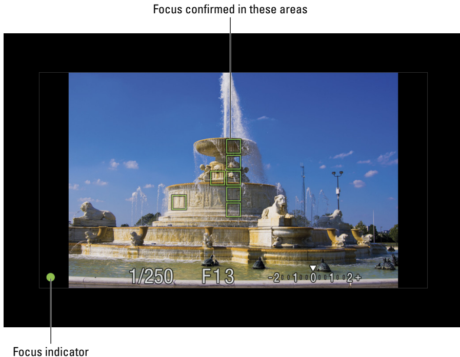
Figure 8-1: The green dot and green squares tell you that auto focus has been successful.
